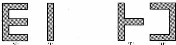
Fig 1. Typical shapes of laminations from which conventional power transformer cores are usually built up, including a gap
